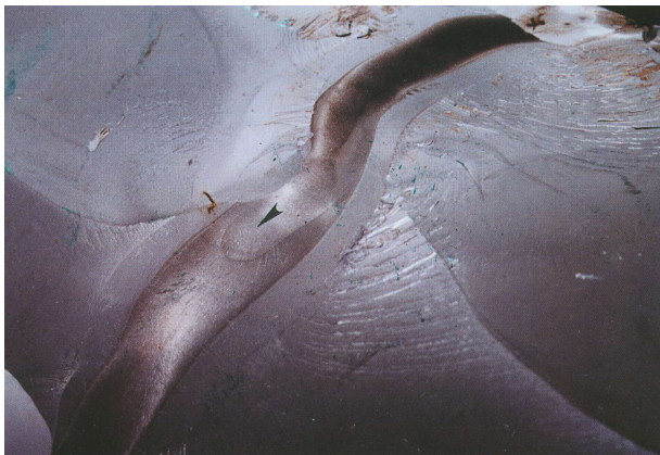
Photo-1- spalling due to surface originated defect
