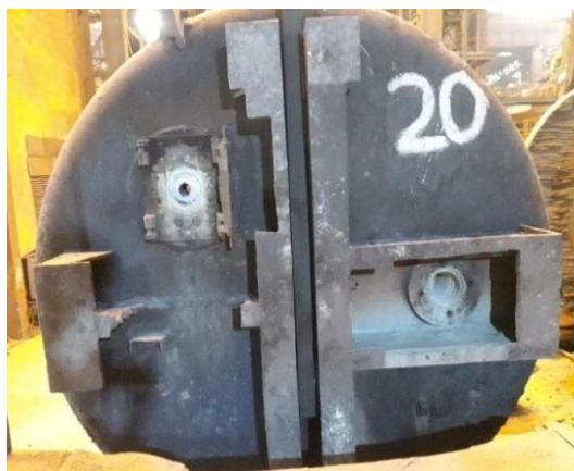
Figure 5: Steel Ladle with Single and Double Porous Plug
