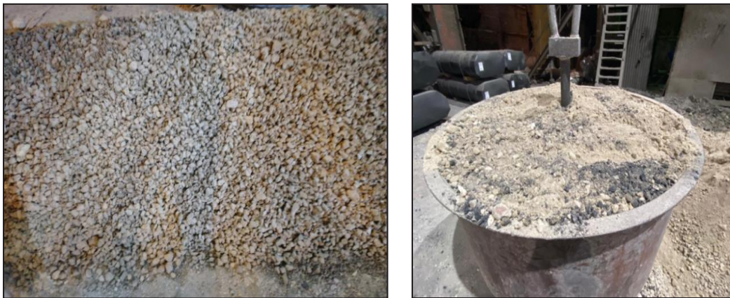
Figure 6: Limestone Chips (–30 mm) Used in Foamy Slag Practice
