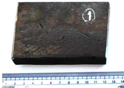
Figure 4: Photograph of the as Received Steel Plate Sample of 25 mm Showing Defective Region
