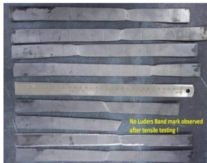
Figure 10: Pictures of post tensile test samples without Luder's band marks
