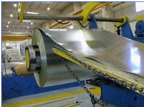
Figure 1: A Coil with Edge Waviness
