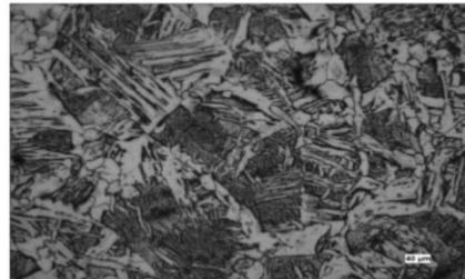
Mag: 500X, Microstructure not acceptable
