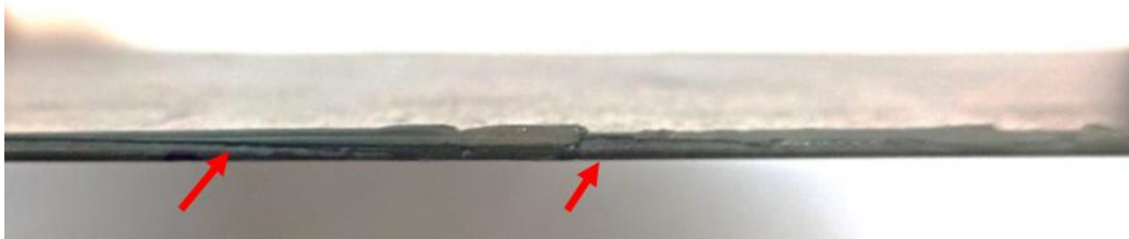
Figure 5: Stereo Graphic Projection of the Double Slit Edge in Hot Rolled Coil
