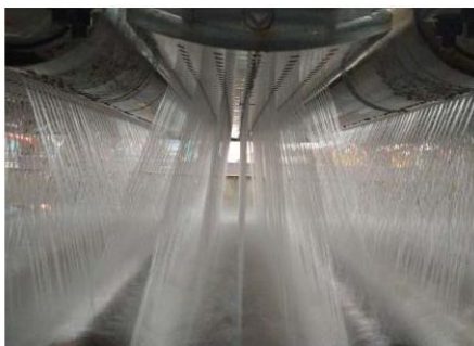
Figure 8: Inclined Jet Pattern in ADCOS [1]
