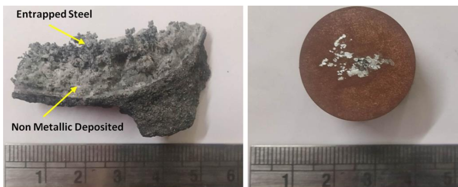
Figure 3: The SEN Clog Material (indication of entrapped steel) and Mounted Sample of Clog Material
