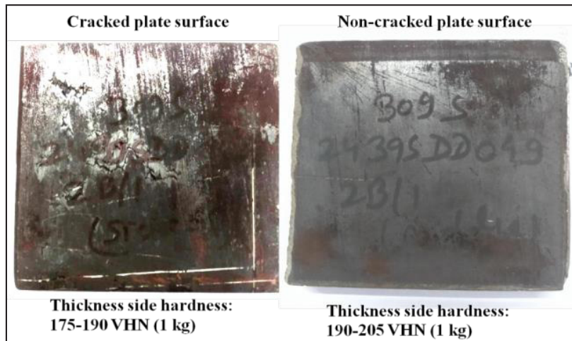
Figure 1: Macro Surface of the Cracked and Non-cracked Samples of the Failed AISI 309S Austenitic Stainless Steel Plates
