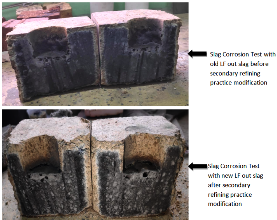
Figure 11: Slag Corrosion Test of Slag Zone Brick with Old and New LF Out Slag
