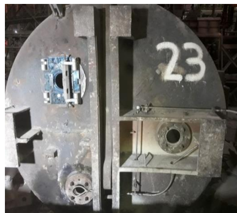
Figure 5: Steel Ladle with Single and Double Porous Plug
