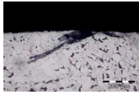
Figure 5: Optical micrographs of the steel plate in 2% nital etched condition showing decarburization along the upper half of the entire length of the transverse cracks and at the crack mouth; (a) 200X Mag.
