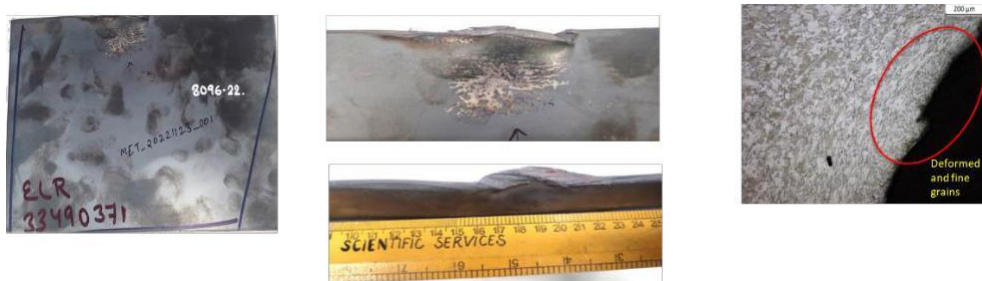
Figure 7: Edge Crack Defect Metallography
