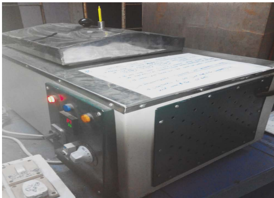
Fig 5 Pictorial view of the constant temperature oil bath
