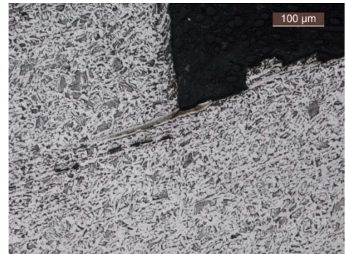
Fig 8 - No segregation line was observed under normal 3% nital etching.
