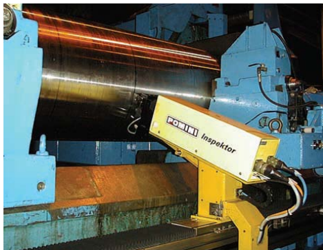
Fig: Eddy Current and UT inspection system to accurately measure surface and sub-surface roll defects
