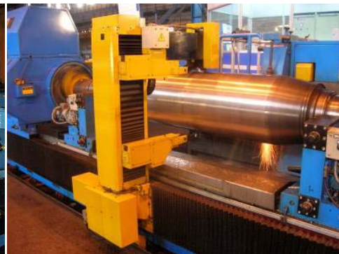
Fig: Independent caliper for 100% roll inspection during grinding
