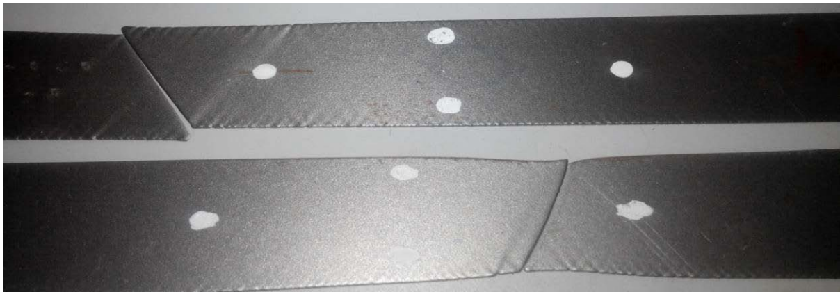
Fig 2 Ludder Band marks on the tensile sample
