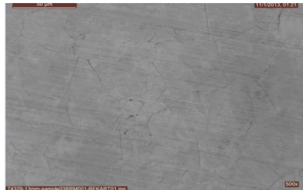
Fig 2 Grain boundary carbides in spring
