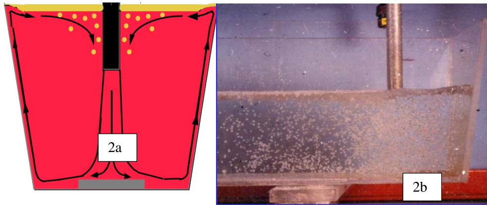
Fig 2a) Schematic of the Tundish slag emulsification, Fig 2b) A water model of tundish depicting the slag emulsification at the pouring area.
