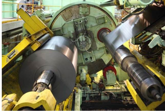
Fig.11: Carousel Coiler at the delivery section
