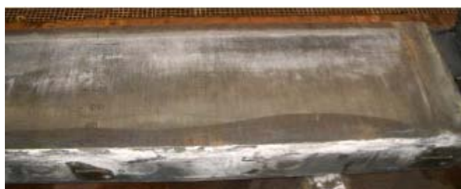
Fig 7 Typical bottom wear at a slab mould, related to friction and cavitation effects
