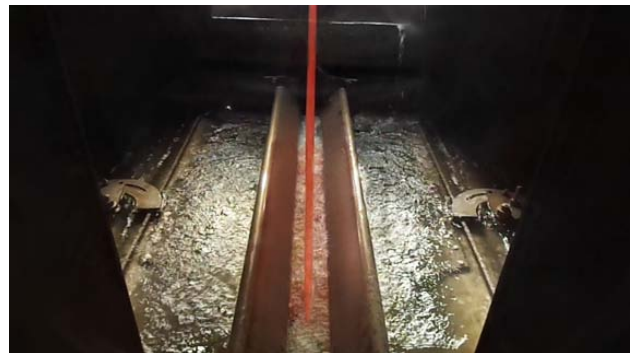
Fig 8 Water-spray cooling for producing steel grades with tensile strengths of up to 1,700 mega Pascal
