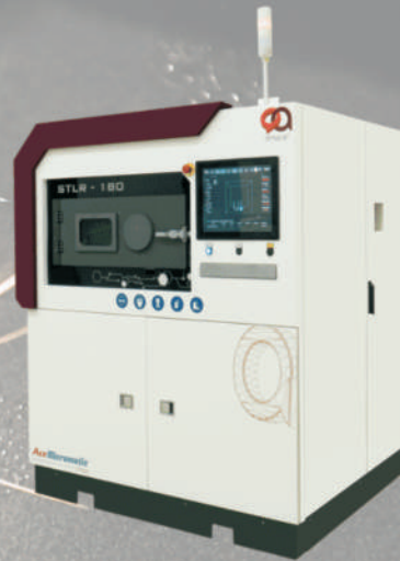
STLR 180 Build envelop Ø180mm x 175mm
