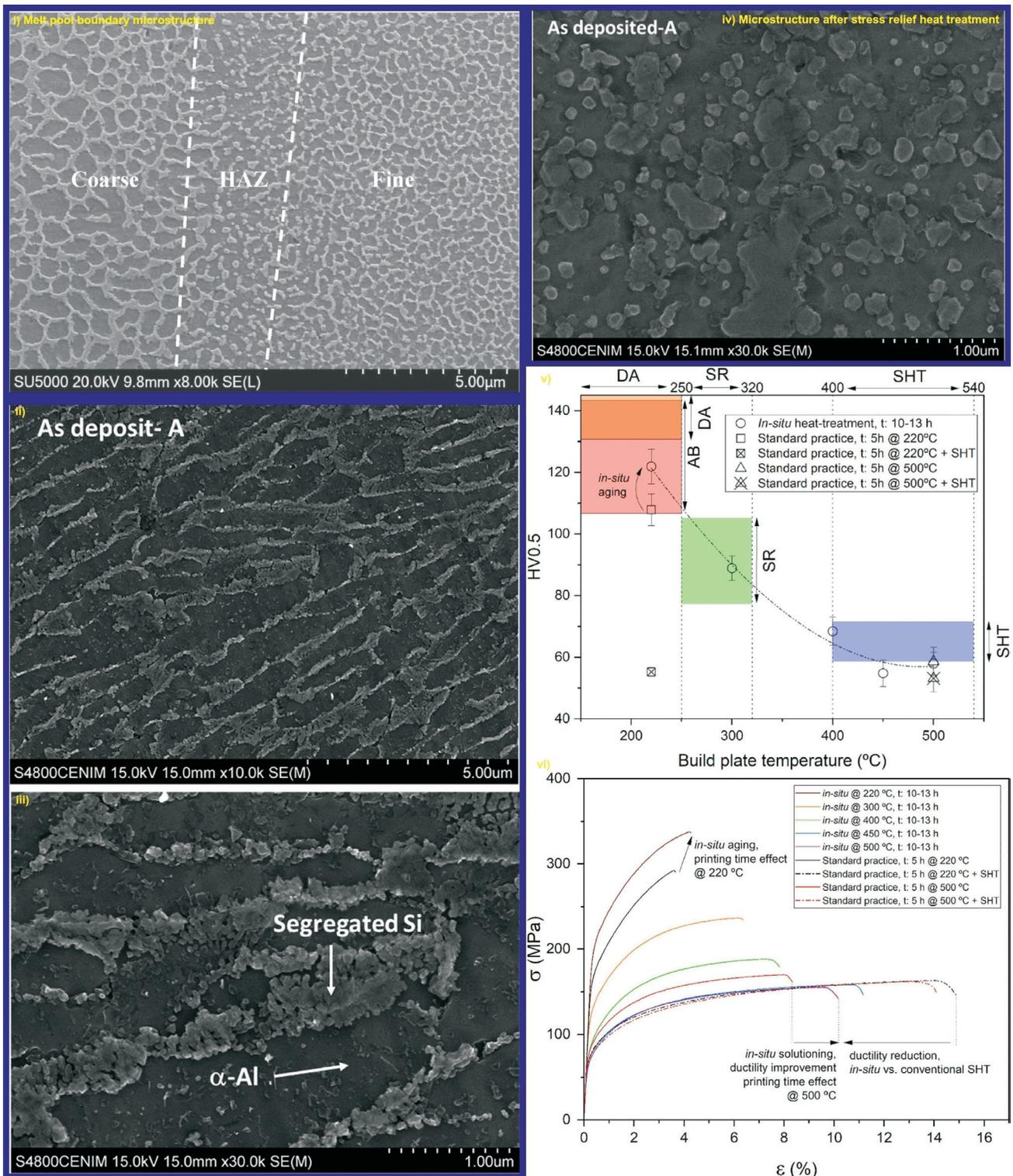
**Fig. 4: i) Melt pool morphology of AlSi10Mg alloy depicting HAZ [38] ii) and iii) depicting the as built eutectic microstructure in further detail and iv) evolution of microstructure with stress relief heat treatment at 573 K for 2 hours [39] v) Effect of heat treatment on microhardness and vi) Effect of heat treatment on tensile properties [40]. Reproduced with permission from Elsevier under Creative Commons Attribution license 4.0**
