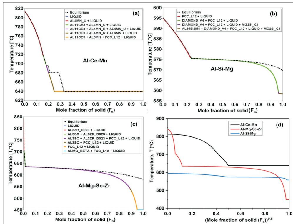
**Fig. 2 : T- $F_s$  curves for various alloy systems generated through Schiel — Gulliver Solidification modelling. Reproduced with permission from Elsevier under Creative Commons Attribution license 4.0 (CC BY-NC-ND)**
