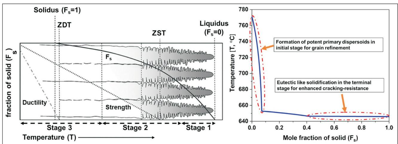
Fig. 1 : (a) Schematic illustrating the dendritic solidification through temperature ( $T$ ) - fraction of solid ( $F_s$ ) plot and b) strategy to enhance printability of Al alloys through computational approaches that predict  $T$ - $F_s$  curve. Reproduced with permission from Elsevier [7] under Creative Commons Attribution license 4.0 (CC BY-NC-ND)
