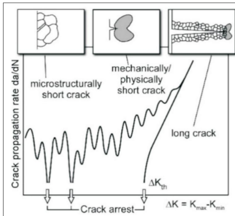
**Fig. 6 : A schematic illustration of proliferation of fatigue cracks in engineering materials [47]. Reproduced with permission from Elsevier under Creative Commons Attribution license 4.0**
