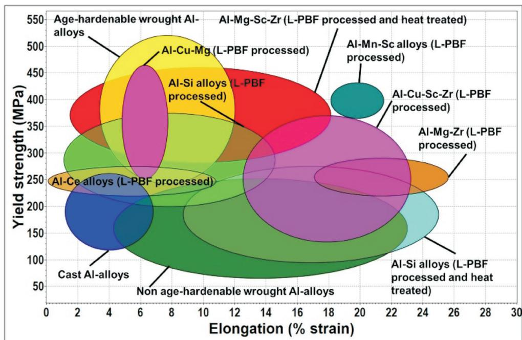
Fig. 5 : Ashby plot depicting the room temperature tensile yield strength and elongation of Al alloys [7]. Reproduced with permission from Elsevier under Creative Commons Attribution license 4.0 (CC BY-NC-ND)
