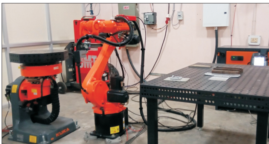
Fig. 4 : A photograph showing WAAM facility with Robot, CMT system and controller.
