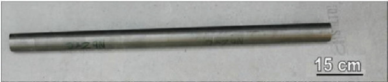
Fig. 6 : Tubular product of Nb alloy obtained using low temperature deformation flow sheet.
