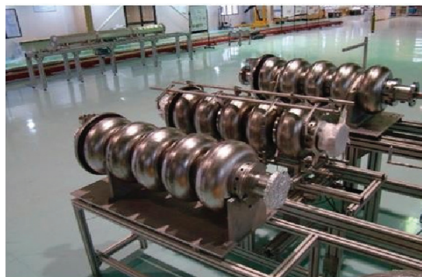
Fig. 2 : Vacuum cavities prepared in DAE and provide US national labs for accelerators.
