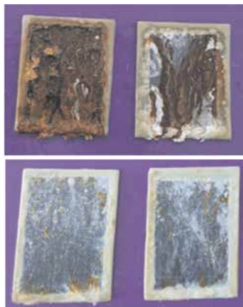
Fig. 11 : Comparison salt fog exposed coated panel (a) plain zinc coating and (b) Zn-0.02Sr Coating.
