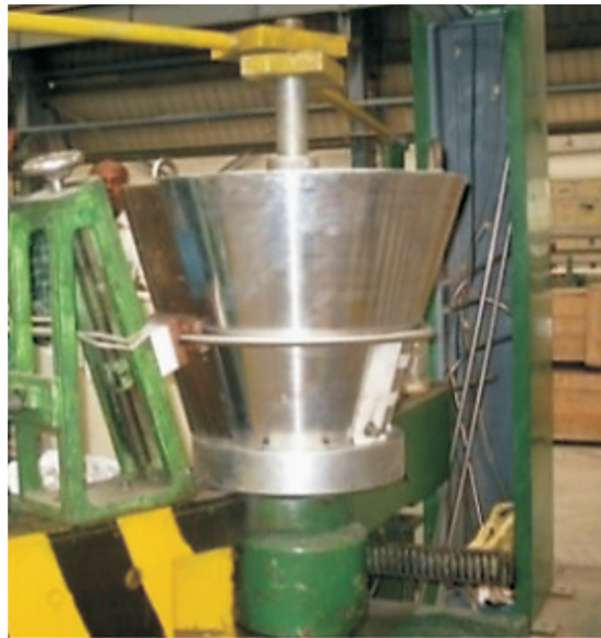
Fig. 6 : U bending over Conical dies
