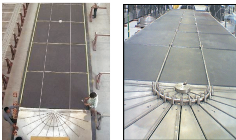
Fig. 9 : Surface Plate Gauge Block for U bend tubes
