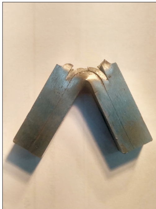
Fig. 2 : Photograph showing the symmetry of anvil trace with respect to notch of the tested CVN specimen.
