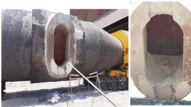
Condition of torpedo spout after preheating
