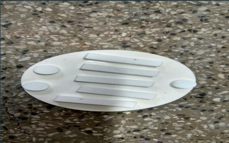
Pellet after sintering at 1200°
