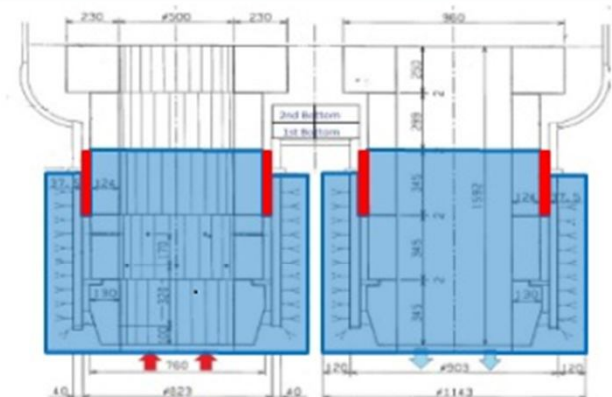
Step 3: Installation of Free flow castable
