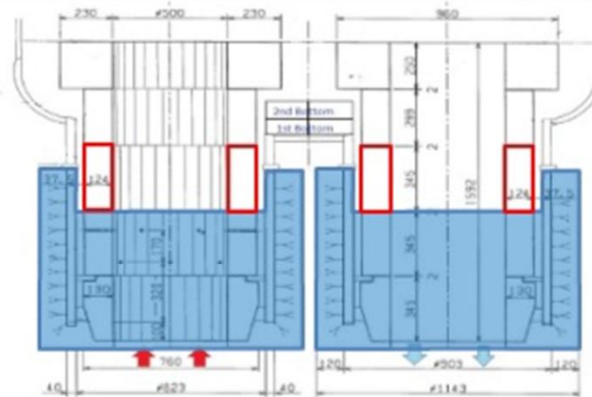
Step 2: Installation of 3 rd Ring Bricks, max 2 mm Mortar. Gap between shell - 20-35 mm. (if not- Report)
