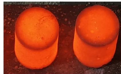
Fig.2 Appearance of DBMC brick after Spalling
