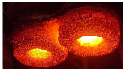
Fig. 15: Appearance of Snorkel after 31 st heat
