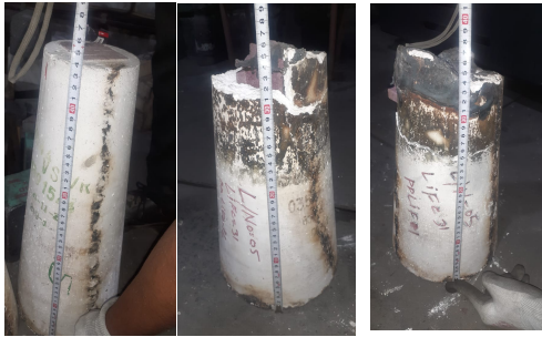
Fig 4: Remnant plug thickness measurement (New vs Used)
