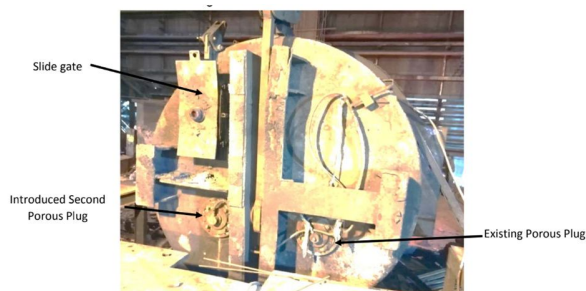
Figure 8: Bottom view of modified ladle
