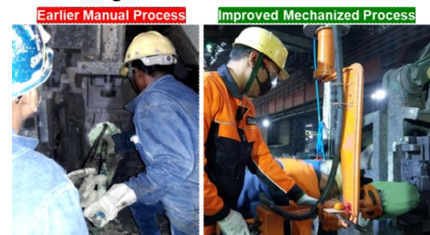
Fig. 10 Fixing of upper nozzle manual & mechanized way
