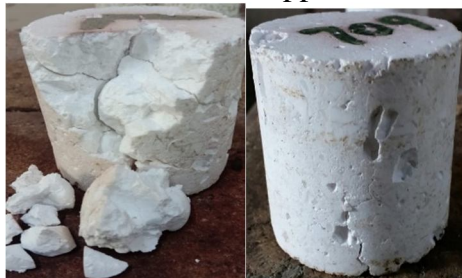
Fig. 7. Thermal spalling test after 26 cycles
