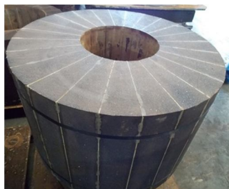
Fig. 11: Final appearance of brick ring
