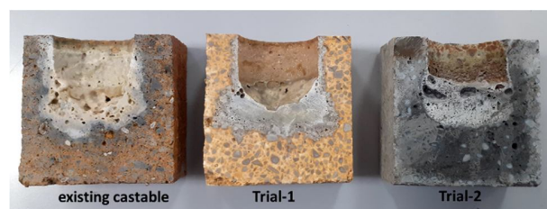
Fig.9: Corrosion test with BF slag after firing at 1500 C/ 3hrs
