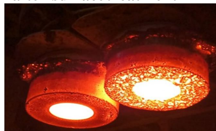
Fig. 14: Appearance of Snorkel after 1 st heat
