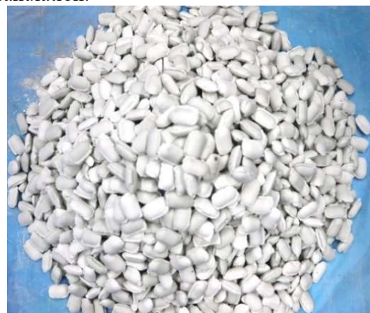
Fig. 1: Sintered high alumina aggregates (briquettes) prepared from sillimanite beach sand.
