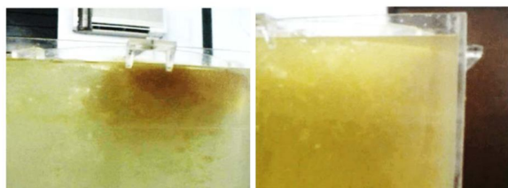
Figure 7: Slag-metal intermixing: Single Porous Plug (Left), Double Porous Plug (Right)
