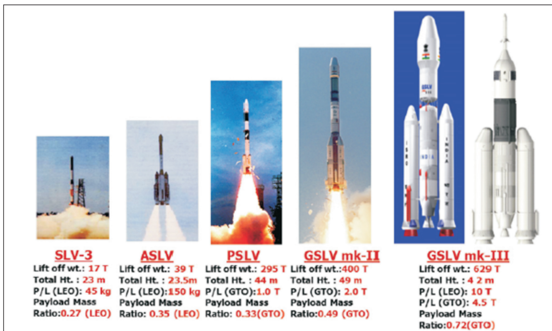
Fig. 1: Progress in ISRO's satellite launch vehicle development program during the past five decades. Both SLV-3 and ASLV used predominantly steels for their construction and are based on solid propellants. PSLV second stage and GSLV, both Mk-II and Mk-III versions extensively use Aluminum alloys for earth-storable and cryogenic propellant tanks. The far right picture shows the GSLV MkIII (LVM3) with Gaganyaan configuration. The complexity of materials technologies increases from left to right.
