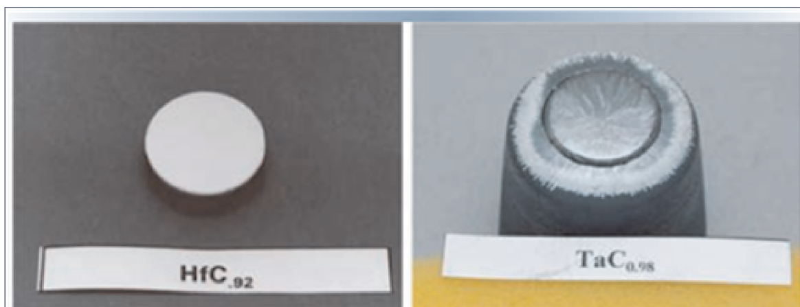
Fig. 11 : Optical micrographs of HfC and TaC after 3 minute exposure at T > 2000\text{ }^\circ\text{C} [14]
