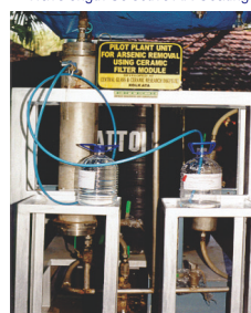
Pilot Plant for Arsenic Removal
