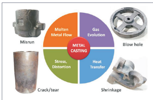
Fig. 2 : Major casting defects related to process
