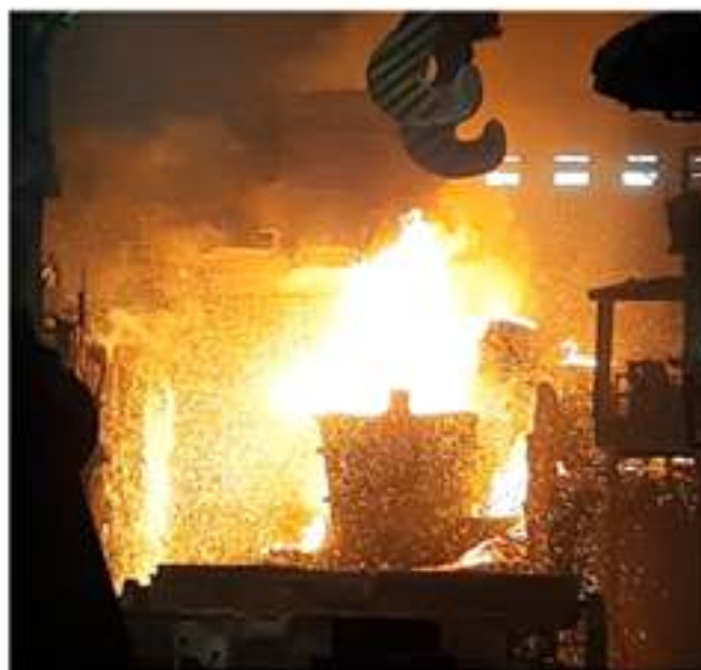
Fig 4: SN mechanism Leakage
