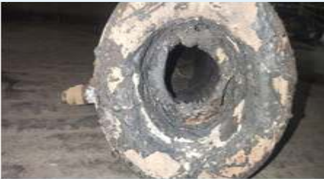
After 10 th Heat, LS changed due to Neck Puncture
