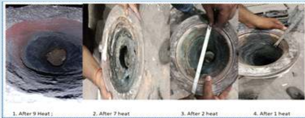
Some Snapshot -- Neck Condition – No Such Erosion Observed
