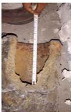
Horse Shoe Crack After 2 nd Heat, From exit bore 210 mm to 230 mm . Metal dipping zone.
