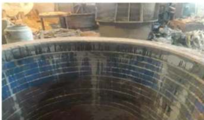
Samwha Lip- Locking Bricks Ladle In Operation (FB is very Robust even during Frequent hard Lip jam removals)
