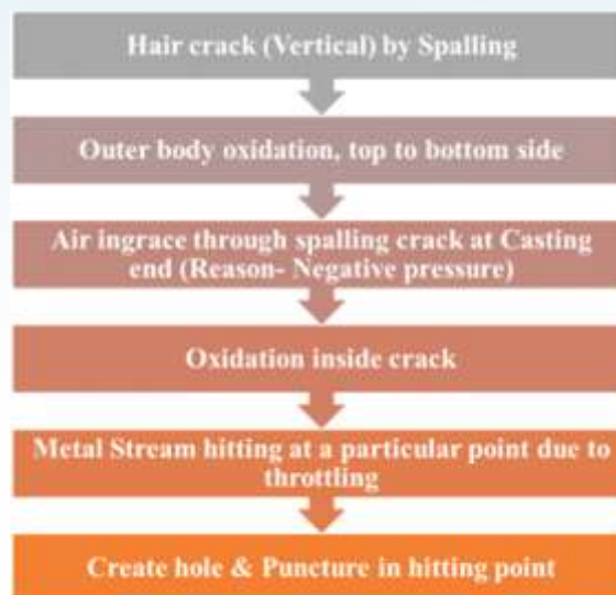
Fig 16: Chronology of lower nozzle puncture
