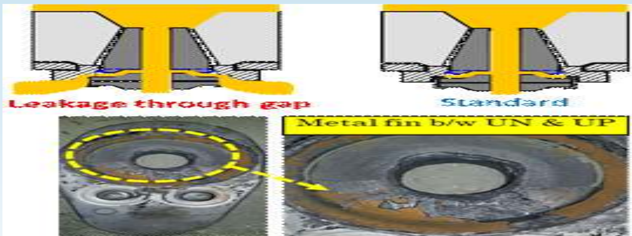
Fig 7: Gap creation and leakage mechanism
