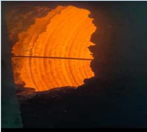
Fig-4 Condition of the ladles without addition of synthetic slag
