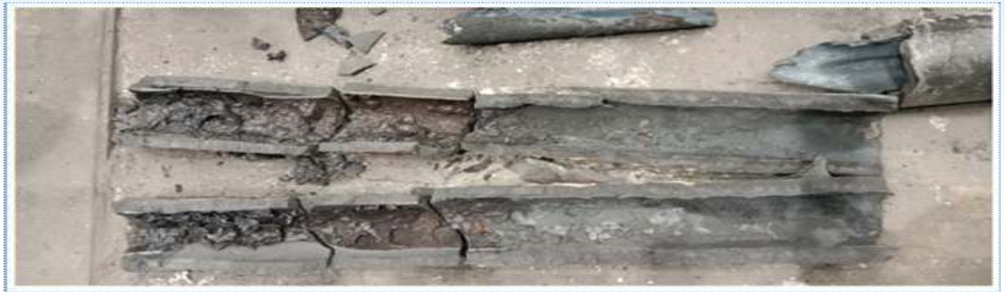
Some Snapshot -- Barrel Part Condition After 9 Heat
