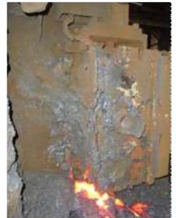
Fig 11: Leakage from SN mechanism
